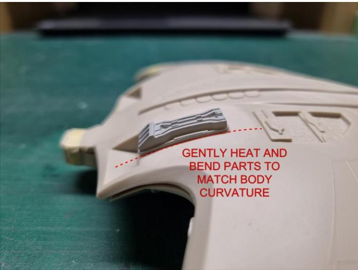
The “mechanical foot” part needs to be bent slightly to match the curvature of the lower hull contour.
