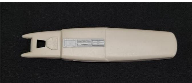
The nacelle detail is shown in some reference photos of the original filming model but missing in others (screengrabs etc). It's likely that this detail is only present on one side of the filming model. I've included 2 parts, so the choice is yours!
